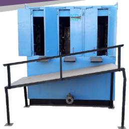
With the help of this plant, one can take on line production, designed in such a way can load drums in 3 rows from front side with the help of hyd. device. Each row containing series of no. of drums in line. Empty drums exit from rear side of Plant.
